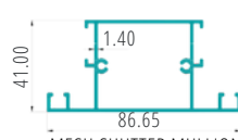
MESH SHUTTER MULLION Wt./R.Mtr. : 1.147 kg PART CODE:27045
